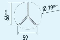
The Beefy profile has 230% more strength than the standard post with a 60% greater surface area providing far better ground adhesion.
